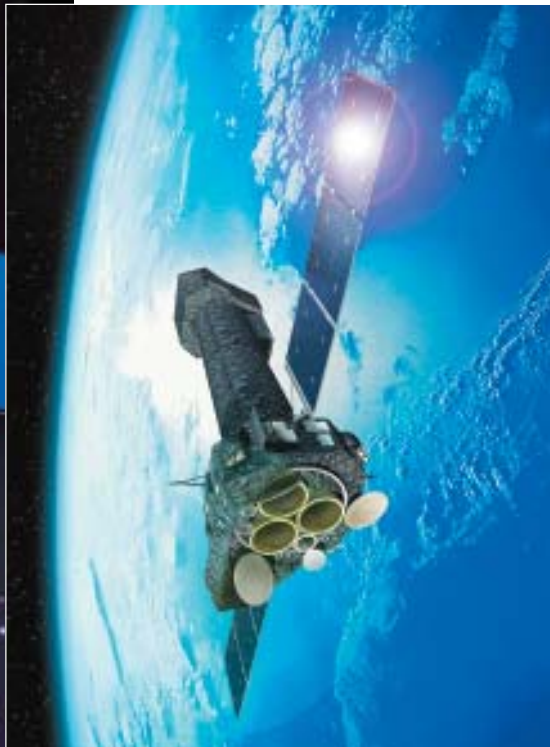
ESA's XMM-Newton X-ray telescope used over 170 wafer-thin cylindrical mirrors spread over three telescopes. ESA
