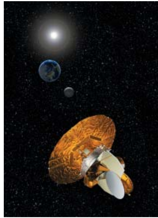
WMAP used the Moon to gain velocity for a slingshot to the L2 Lagrange point, one million miles (1.5 million km) beyond the Earth.
